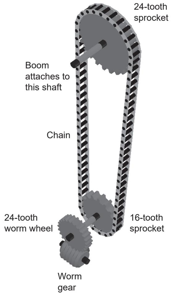
The length of the boom from the centre of its attachment shaft to its tip is 3.25 m. The boom normally rests in a horizontal position, as shown in the diagram on the right. When it opens, it rotates in an arc to its fully open position, which is 90° vertical. At full speed, the tip moves at 1.021 m s<sup>-1</sup>.
